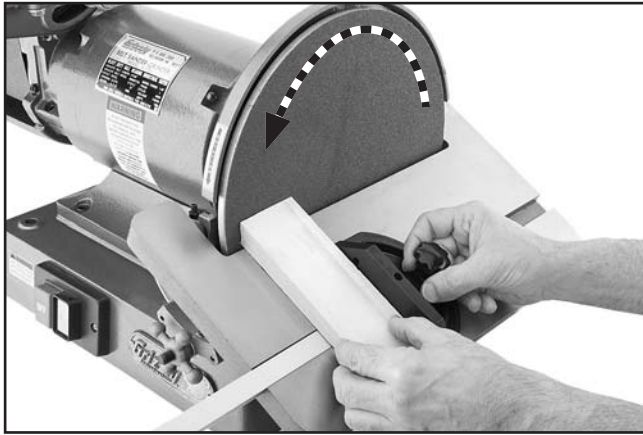
Figure 34. Example of compound angle sanding.
